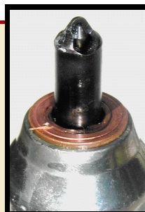
This injector failed due to contaminant exposure. Note the damage to the tip.
